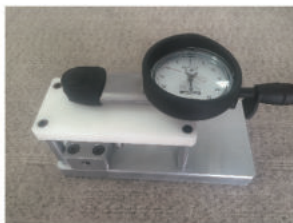
Screw head torque test 螺丝扭矩测量
